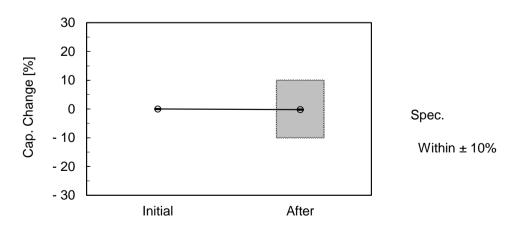
(Dielectric Strength) AC4000V(r.m.s.),60 s Dielectric Strength (Between lead wires) : No failure Dielectric Strength (Body Insulation) : No failure Insulation Resistance (I.R.) :  $1000M \Omega$  min. Appearance : No marked defect
